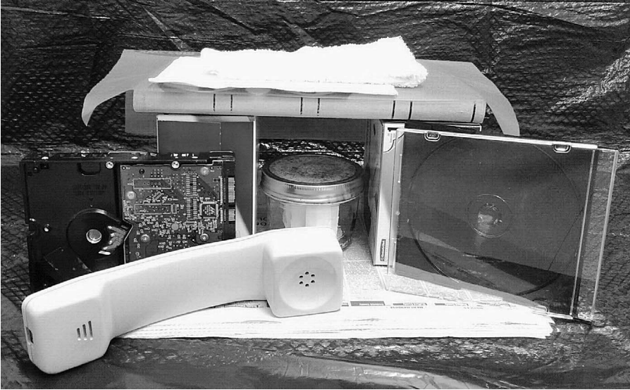
Fig. 2. Trash bag experiments. Cutaway of the contents of a trash bag used in fumigation experiments. Mixed stages and sexes of bed bugs were placed in a wide-mouth canning jar with fan-folded filter paper as a harborage. The jar had a fine nylon (100-mesh) cover and was surrounded with representative items that could not receive a liquid treatment (see Materials and Methods for actual contents). Test compounds were applied to the top cloth and the bag was sealed with tape. The bag was opened 5 d posttreatment, at which time bed bug mortality was assessed.
