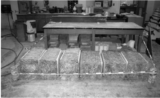
FIGURE 4. Completed plastered bales.
