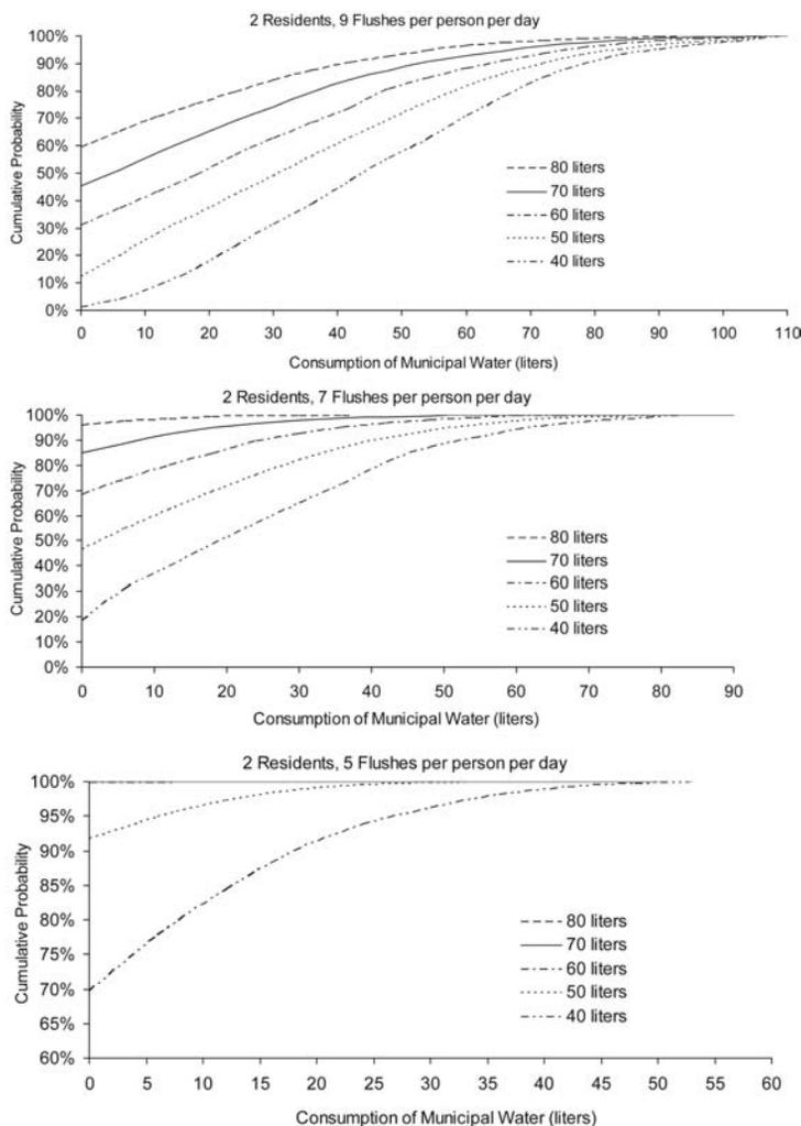
**FIGURE 3.** Cumulative probability for the volume of municipal water consumed when the graywater system in Figure 1 is equipped with two tanks of the indicated size. There are 2 residents, each of whom flushes the toilet 5, 7 or 9 times per day.
