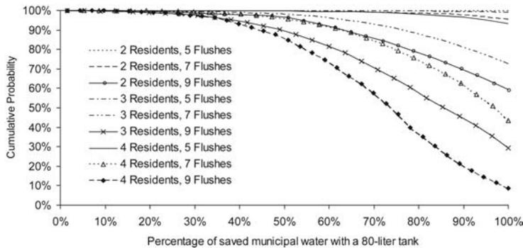
**FIGURE 6.** Percentage of municipal water saved when the graywater system of Figure 1 is equipped with two 80-liter tanks.
