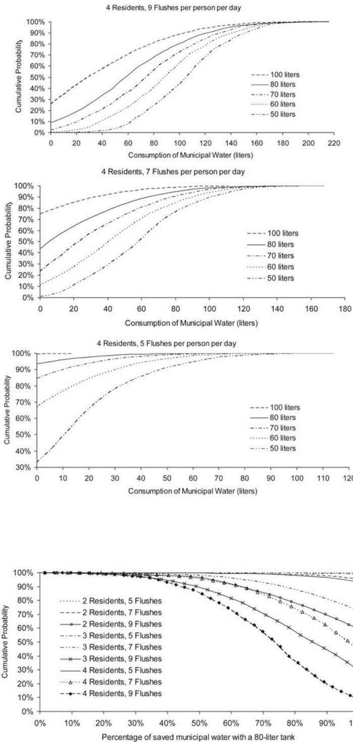
**FIGURE 5.** Cumulative probability for the volume of municipal water consumed when the graywater system in Figure 1 is equipped with two tanks of the indicated size. There are 4 residents, each of whom flushes the toilet 5, 7 or 9 times per day.
