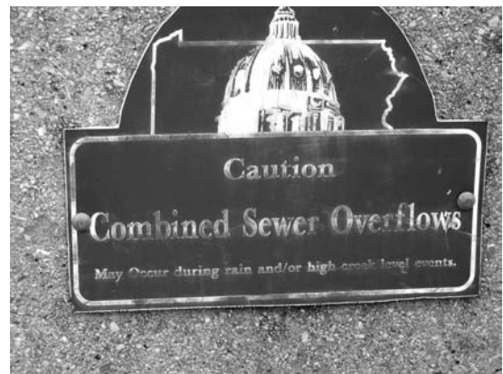
FIGURE 15. A warning sign near a CSO outlet in Harrisburg, Pennsylvania. Combined sewer overflows are among the earliest sewer systems and were designed to carry both stormwater and sewage to a treatment plant. However, in large storms the flow capacity of these systems can be exceeded and the overflow is dumped directly into water bodies. The overflow often contains untreated municipal wastewater, raw sewage, industrial waste, debris, and other pollutants, and it poses a major threat to human health and the environment. (Photo courtesy of Christopher J. Sutton, Western Illinois University.)
