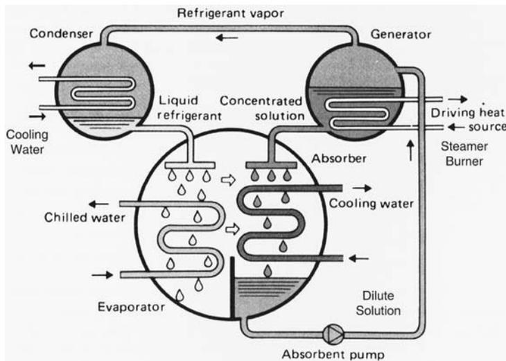
**FIGURE 3.** A chiller-heater operates via direct-fired, two-stage absorption units that use water as the refrigerant and lithium bromide as the absorbent. (Diagram courtesy of York Air Conditioning Systems.)
