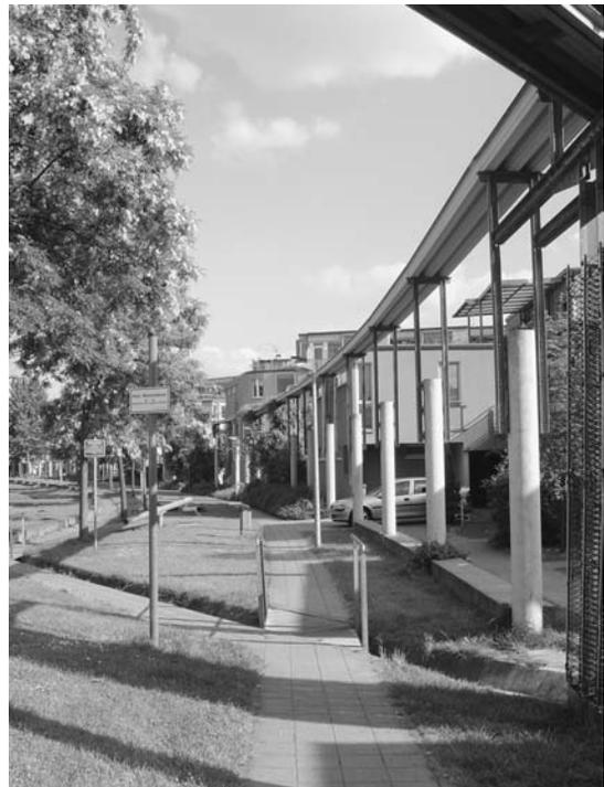
**FIGURE 4.** Central green water retention and infiltration zone, Koppersbusch, Gelsenkirchen, Germany.
