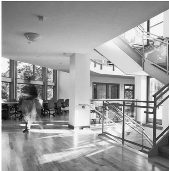
**Maximize natural light.** Daylighting strategies were employed to both minimize lighting loads and provide an excellent indoor aesthetic environment throughout the facility (Figure 3).
