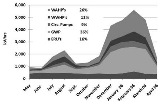
During the heating-season months of October to February the enthalpic-energy-recovery ventilation system recovered 11,700 kWh-t while using 3,800 kWh of electricity, resulting in an estimated Coefficient of Performance (COP) of -3.1.
