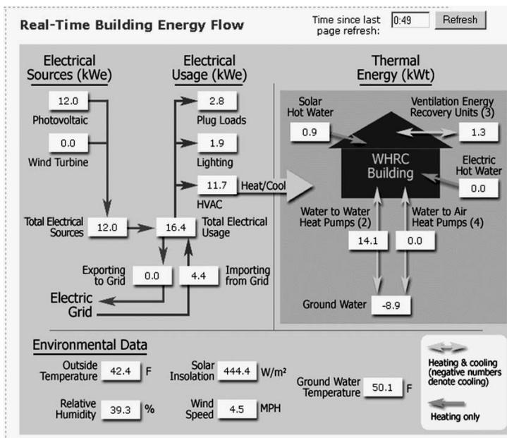
**FIGURE 8.** A snapshot of energy flows through the Research Centers office facility is displayed in near real time. The Energy Flow page is a schematic overview of the energy flowing through the WHRC facility. <http://www.whrc.org/building/education/EngFlw2.asp>.
