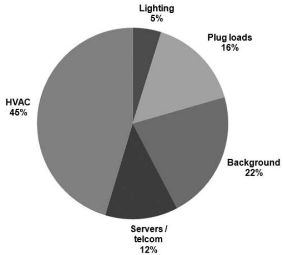
ment and appliance usage from the significant background/parasitic electrical usage of the building. This background electrical load was observed to be approximately 2.4 kW continuous. This was measured while the building was nominally "at rest," with all lights off, and all HVAC and refrigeration equipment shut down at the breaker panel.
