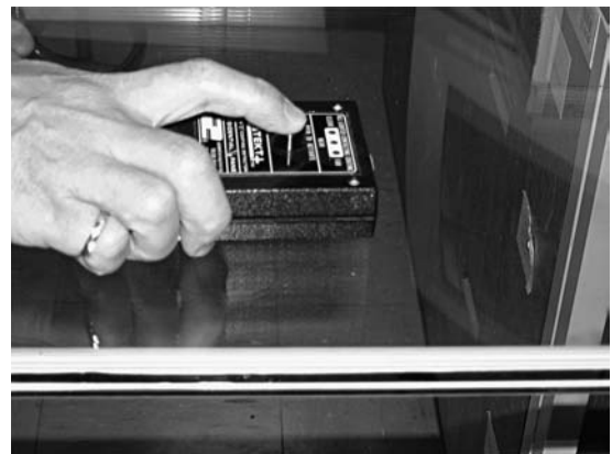
FIGURE 10. Electronic detection of low-e coating
