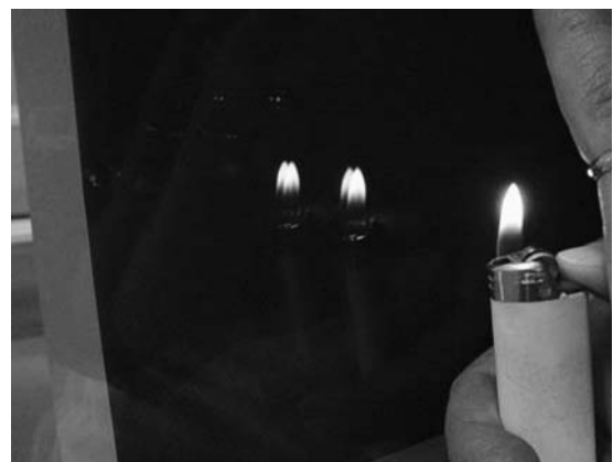
FIGURE 11. Using a light source to check for low-e
