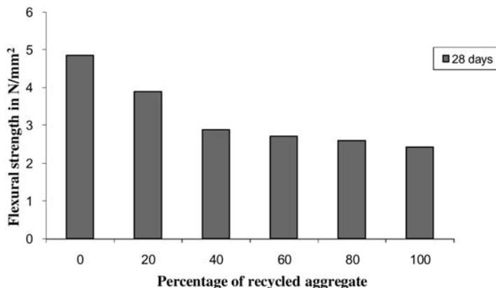
**FIGURE 5.** Effect of RA Content on Flexural Strength.
