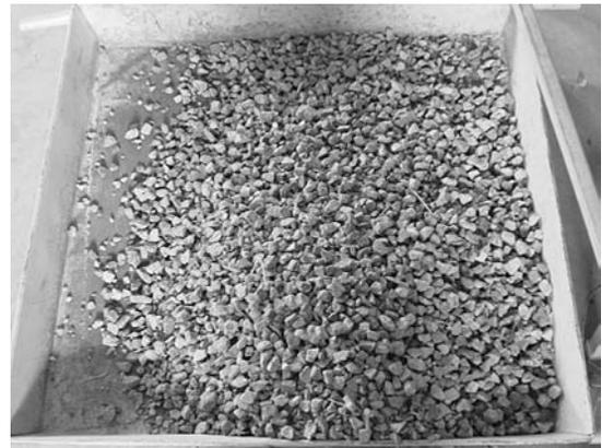
obtained from demolished structures. They were further crushed in the laboratory to produce coarse recycled aggregates passing through a 20mm sieve and retaining on a 4.75mm sieve as shown in Figure 1. Coarse recycled aggregates have a bulk density of 1426.05 kg/m<sup>3</sup> and a specific gravity of 2.63.
