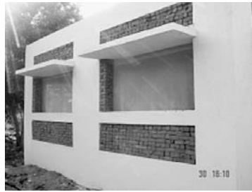
FIGURE 3. Photograph of the experimental model with the fly screen over the opening.
