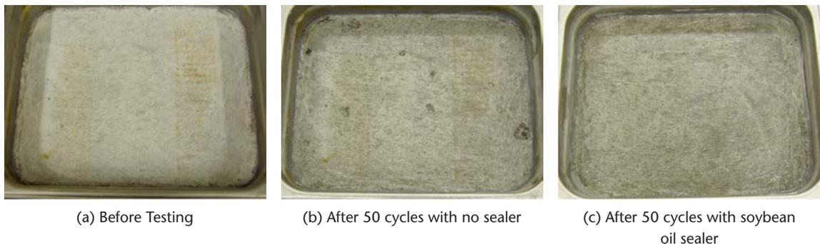
**FIGURE 4.** 50S-VA Deicer Testing Results.
