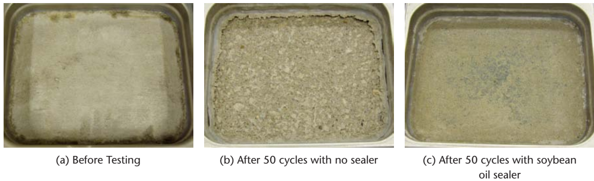
FIGURE 4. 50S-VA Deicer Testing Results.
