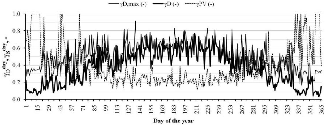
**FIGURE 7.**  $\varepsilon_{\gamma_D}^{\text{day}}$  through the year for a modelled dwelling with (upper graph) and without (lower graph) space heating and domestic hot water (DHW) by means of a heat pump.
