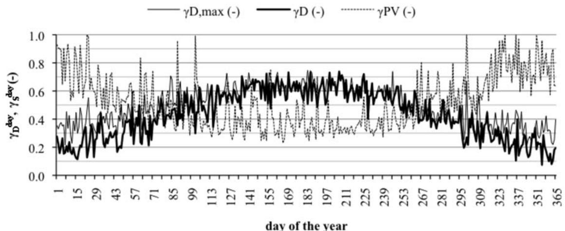
**FIGURE 6.**  $\gamma_D^{\text{day}}$  (bold),  $\gamma_{D,\text{max}}^{\text{day}}$  (black) and  $\gamma_{PV}^{\text{day}}$  (dashed) through the year for a modelled dwelling with space heating but without domestic hot water by means of a heat pump. A resulting  $\gamma^{\text{year}}$  of 0.29 and a value  $\varepsilon_{\gamma_D}^{\text{year}}$  of 0.46 is found.
