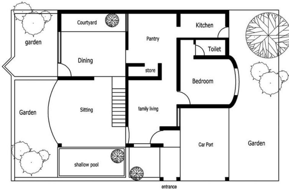
Note: All walls including the boundary wall has been constructed in Compressed Stabilised Earth Blocks
