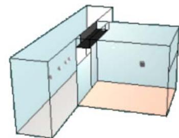
**FIGURE 7.** Vertical transfer-box sections with views from inside and outside of the office. The section of the transfer box is in the right side of the figure. The air exits the office from opening at the bottom of the transfer box (shown as inside) passing through the transfer box and entering the corridor from the top of the box (shown as outside).
