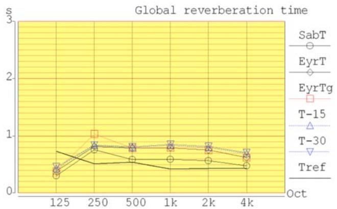
diffuse-field theory (it is shown as SabT in Figure 3) was the reference from the software for RTs. The Tref in the figure represents the measured RT values. The average RTs at the octave-band frequencies from prediction and measurement were similar. It was an indication that the computer model is a good representation of the actual office area.
