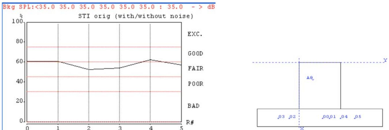
receiver locations along the corridor and one speaker at a typical seating location in the office was considered, as shown in Figure 4. The STI was predicted along the corridor, as shown by numbers from 1 to 5. The X axis represents receiver locations and Y axis represents STIs in %. As can be seen in Figure 4, the various ranges of STI in % (e.g. <30, 30–45, 45–60, 60–75, >75), correspond to different speech intelligibility levels (e.g. BAD, POOR, FAIR, GOOD and EXCELLENT) respectively.
