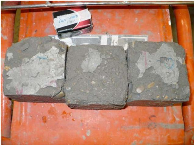
**PLATE 3.** 0.5% Rubber sample at 50 freeze/thaw cycles.
