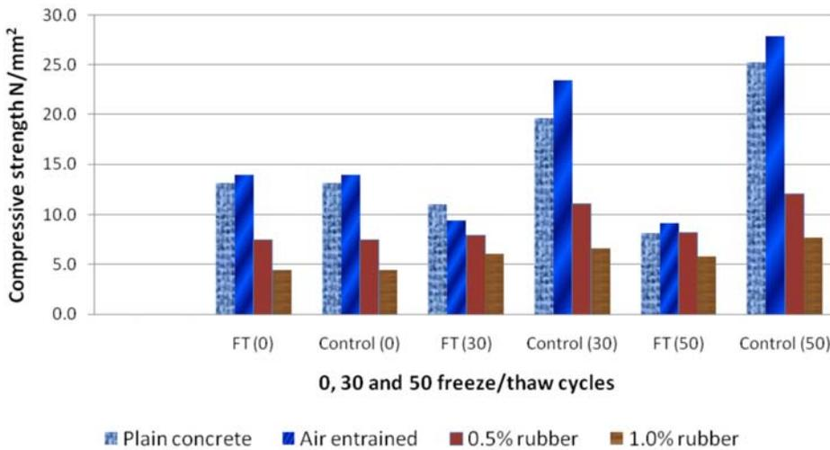
**FIGURE 7.** Freeze/thaw and control sample compressive strengths.
