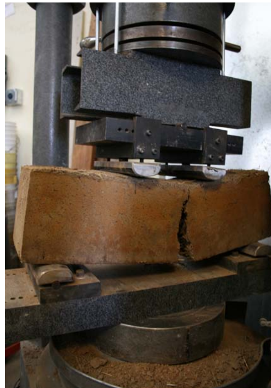
FIGURE 4. Modulus of rupture test setup.
