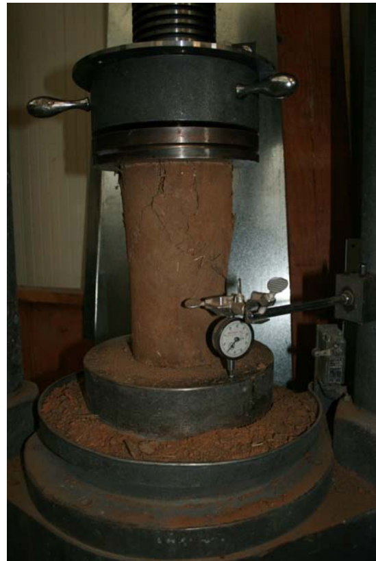
FIGURE 5. Modulus of elasticity test setup.
