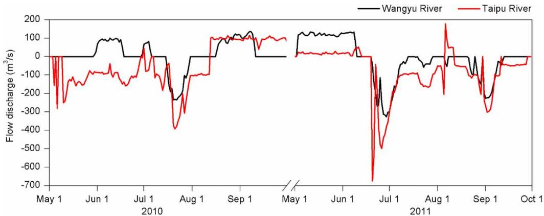
**Figure 4** | The inflow and outflow discharges of the Wangyu and Taipu Rivers between May and September of 2010 and 2011. The positive and negative values represent inflow and outflow river, respectively.
