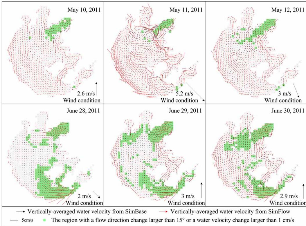
**Figure 10** | The depth-averaged water velocities from two simulations (SimBase and SimFlow) during 28–30 May and 10–12 June 2011. SimBase represents the baseline simulation neglecting inflows and outflows from Lake Taihu. SimFlow represents the simulation considering the water transfers from the Wangyu and Taihu Rivers. The spatial resolution of this figure is adapted to  $1,750 \times 1,750$  m by resampling.
