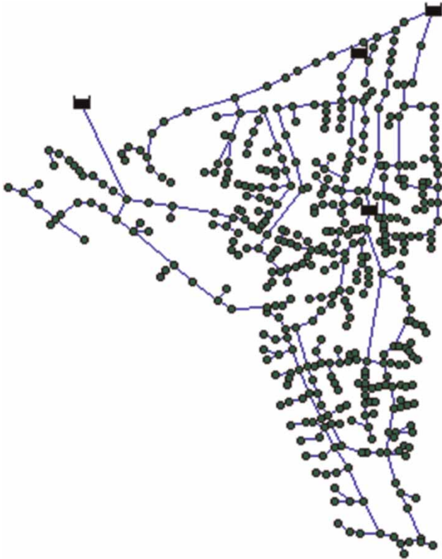
Figure 7 | Layout of the Balerma WDS.
