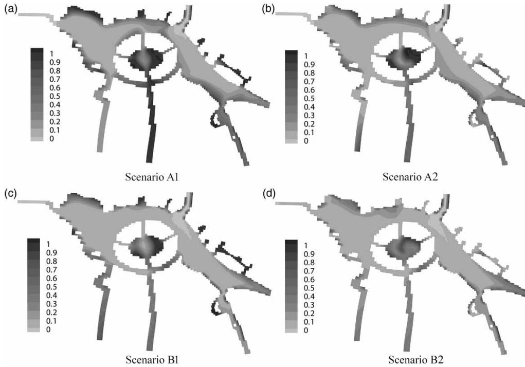
**Figure 6** | Renewal pathways (vertically averaged and plotted at the last day) for: (a) A1, 10 m<sup>3</sup>/s, 30 days; (b) A2, 10 m<sup>3</sup>/s, 30 days, plus pumped inflows at the bays and pumped outflow at the inner lake; (c) B1, 5 m<sup>3</sup>/s, 60 days; (d) B2, 5 m<sup>3</sup>/s, 60 days, plus pumped inflows at the bays and pumped outflow at the inner lake. Light colour represents 'freshwater' with a value of '0' indicating complete renewal.
