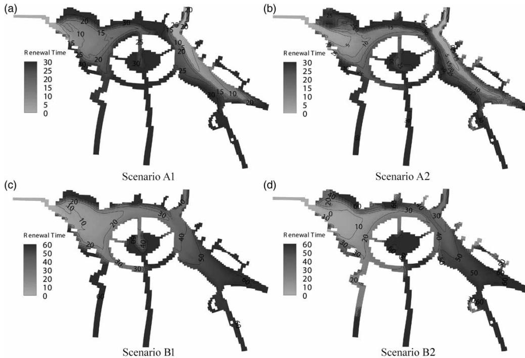
**Figure 7** | Spatial distribution of the LRT within the lake for: (a) A1, 10 m<sup>3</sup>/s, 30 days; (b) A2, 10 m<sup>3</sup>/s, 30 days, plus pumped inflows at the bays and pumped outflow at the inner lake; (c) B1, 5 m<sup>3</sup>/s, 60 days; (d) B2, 5 m<sup>3</sup>/s, 60 days, plus pumped inflows at the bays and pumped outflow at the inner lake.
