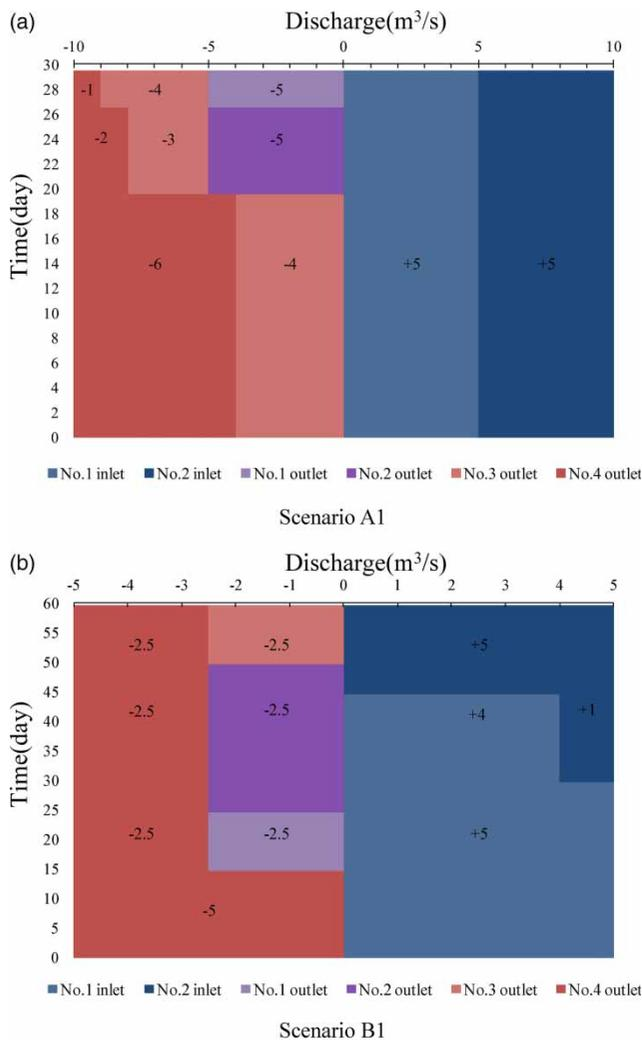
**Figure 4** | Specific model simulation schemes for Scenarios A1 (a) and B1 (b). The total inflow rate equals to the outflow rate. +: inflow rate; -: outflow rate. The corresponding upgraded scenarios contain pumped inflows at the bays and pumped outflow at the inner lake (figures not shown).
