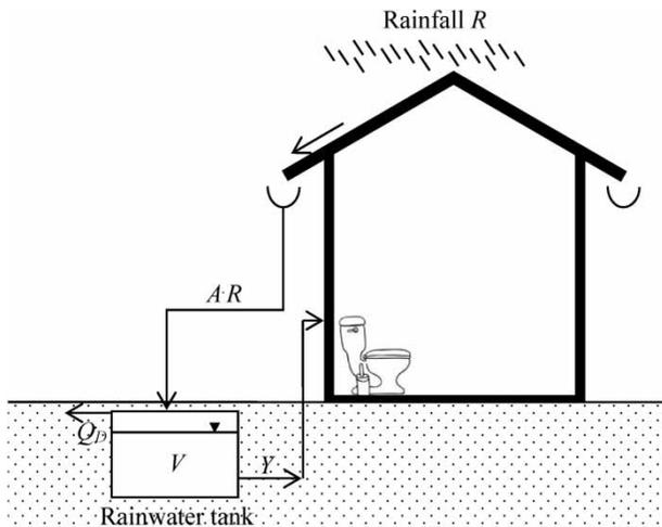
**Figure 1** | Schematic of the domestic rainwater harvesting system.  $R$  is the rainfall,  $A$  is the effective rooftop area for rainwater collection,  $Y$  is the yield from the rainwater tank,  $Q_o$  is the overflow,  $V$  is the volume in store.
