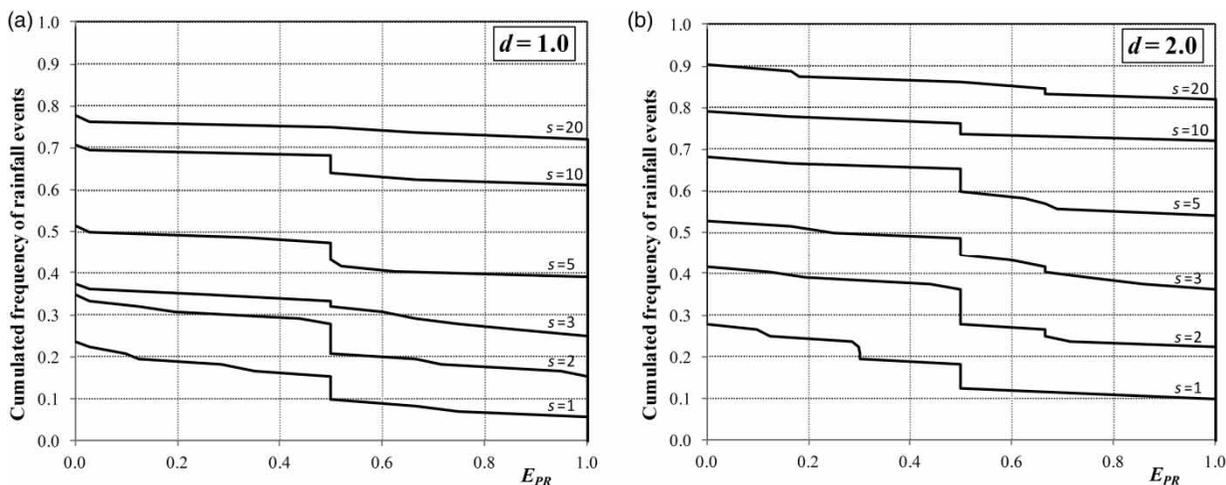
**Figure 6** | Tank peak retention efficiency as a function of the cumulated relative frequency of rainfall events in the year. The household is assumed to host four people. (a)  $d = 1.0$ ; (b)  $d = 2.0$ .
