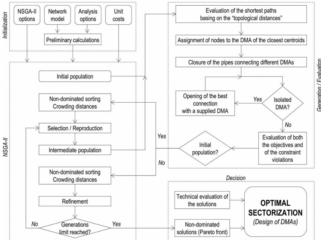
Figure 1 | Schematic of the optimization algorithm.
