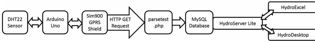
**Figure 2** | Workflow of data from sensor to user.
