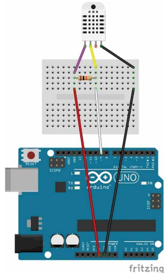
**Figure 3** | Wiring diagram for DHT22 and Arduino.
