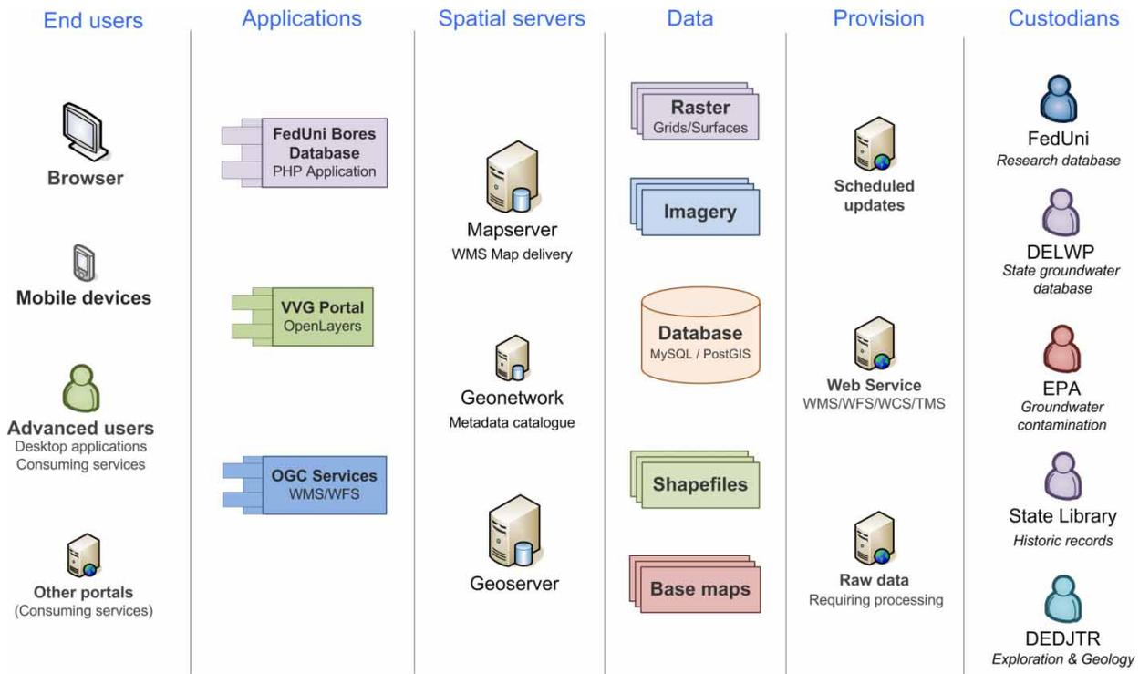
Figure 1 | Generalised systems architecture and data flows for the VVG system.
