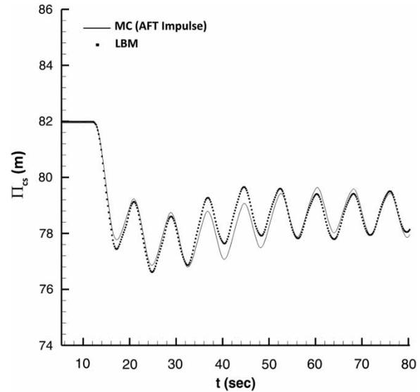
Figure 17 | Hydraulic head, comparison between LBM and MC (AFT Impulse) with an air chamber included.
