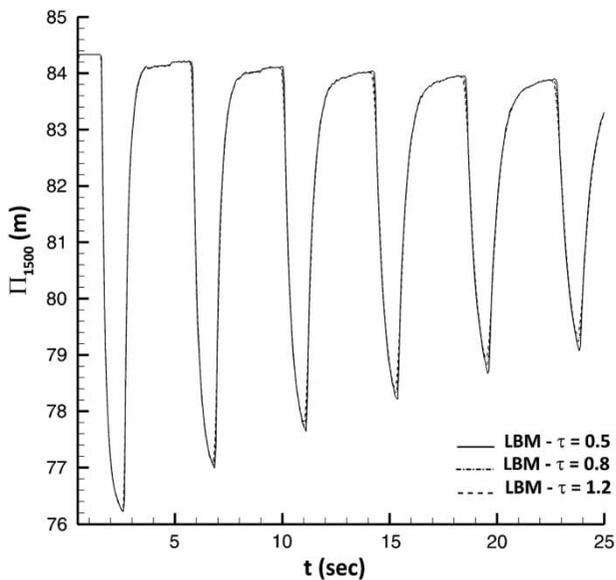
Figure 12 | Dissipation intensity caused by  $\tau > 0.5$ .
