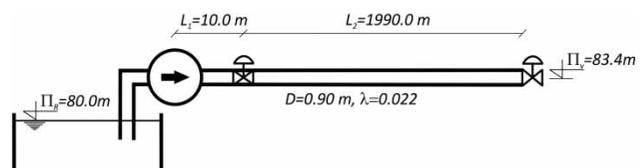
Figure 9 | Single pipeline system.
