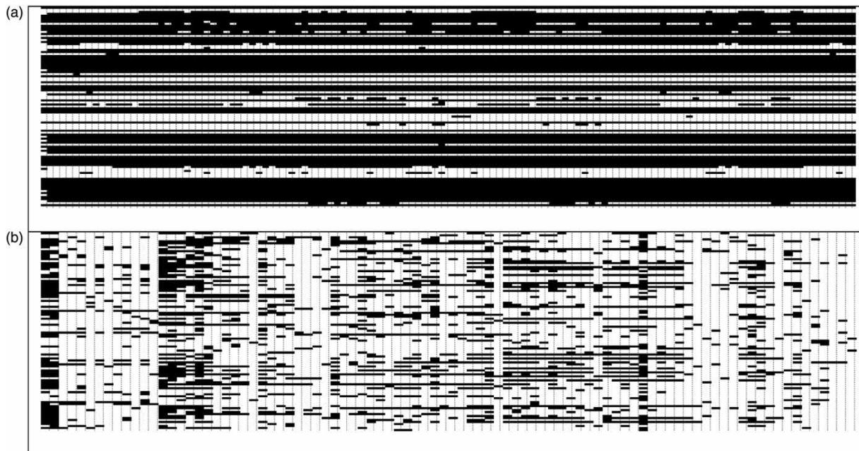
Figure 6 | Detection matrix of (a) pressure meters (100 events (vertical) by 125 nodes (horizontal)) and (b) flow meters (100 events by 90 pipes) with black fill at the cell  $(i, j)$  indicating that the event  $i$  was detected by meter  $j$ .
