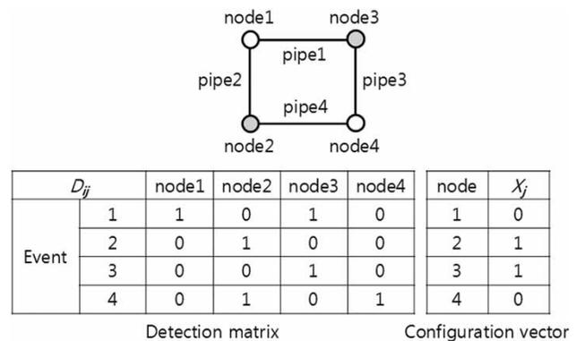
**Figure 1** | The detection matrix and configuration vector of a network (example). Pressure sensors are installed at gray-filled nodes (nodes 2 and 3).
