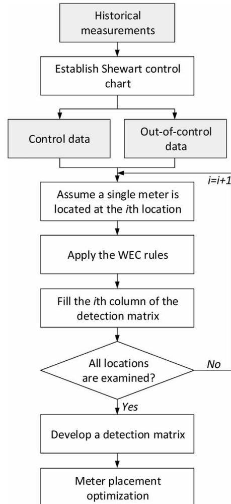
Figure 2 | Flowchart for the proposed optimal meter placement approach.
