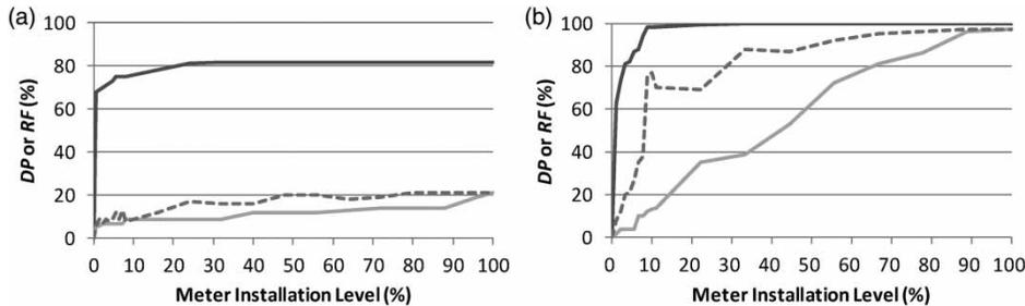
**Figure 18** | ROC curves for (a) pressure meters and (b) flow meters (*DP* (solid black line), *RF* for the best *DP* meter sets (gray dashed line), and minimum false alarm rate (gray solid line)). Note that the total number of pressure meters and flow meters (i.e., meter installation level is 100%) are 125 and 90, respectively.
