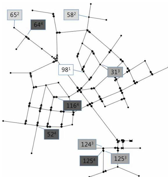
**Figure 14** | Optimal pressure meter locations when one to four meters are installed and  $DP$  is maximized. The value in each box is the node number, with the superscript denoting the allowable number of meters in the sensor network.
