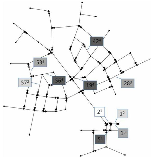
**Figure 15** | Optimal flow meter locations when one to four meters are installed and  $DP$  is maximized. The value in each box is the pipe number, with the superscript denoting the allowable number of meters in the sensor network.
