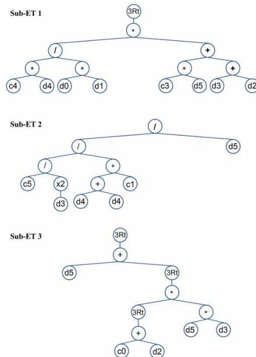
**Figure 3** | Optimal ET structures for the GEP model for prediction of the scour depth around bridge pier with debris accumulation.
