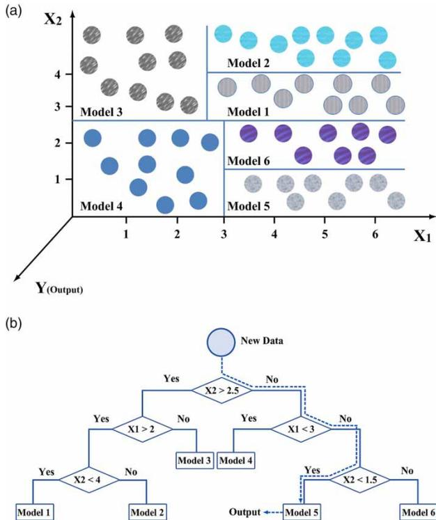
**Figure 4** | Splitting the input space and prediction by the model tree for a new data record: (a) splitting of the input space ( $X_1 \times X_2$ ) by the M5 model tree algorithm; (b) predicting a new data record by the model tree.
