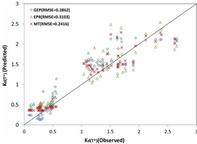
**Figure 7** | Scatter plot of observed and predicted scour depth in live-bed condition for testing of the proposed models.
