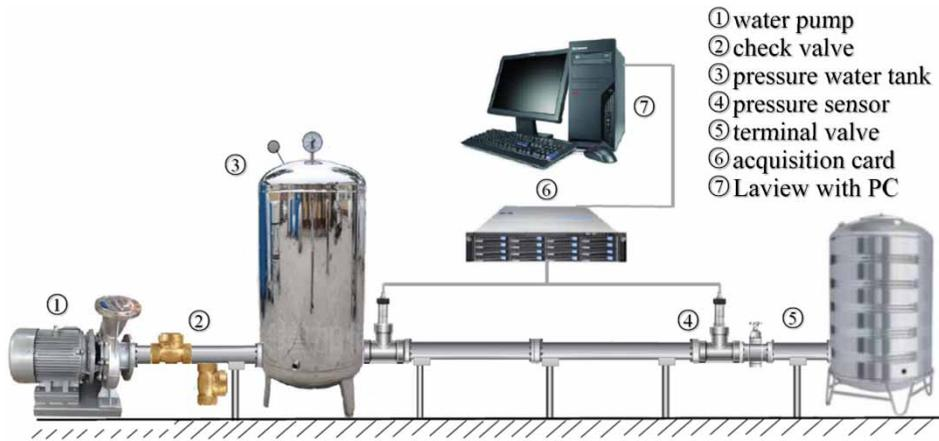
**Figure 3** | Schematic of experimental test system.
