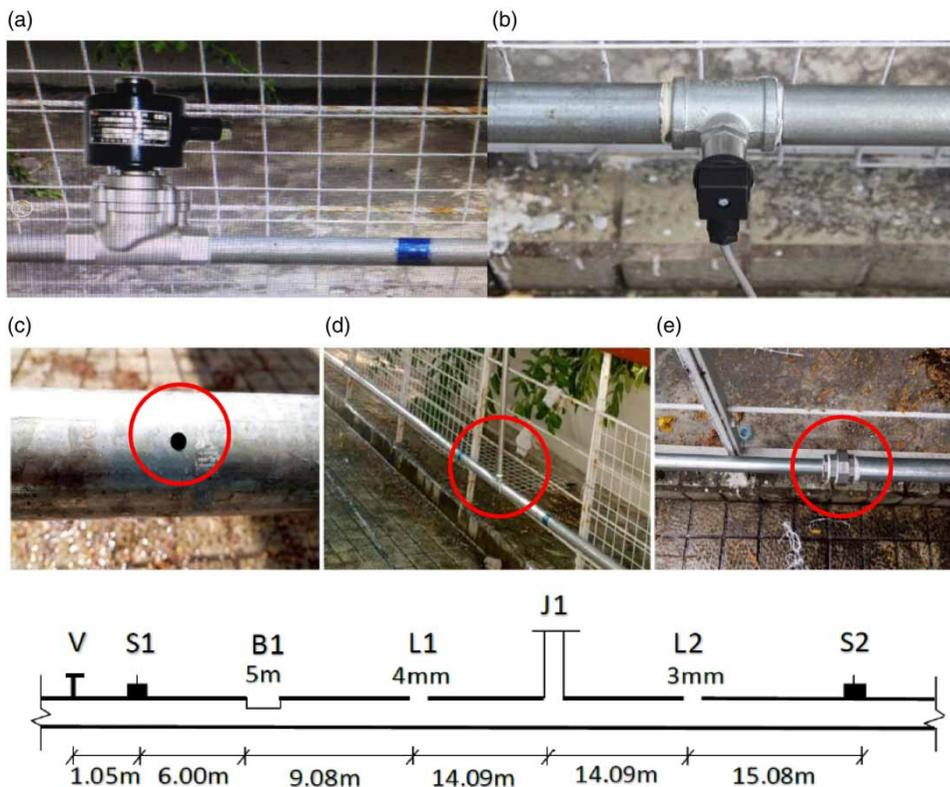
**Figure 4** | Different pipe faults and facilities used for the tests: (a) control valve (V); (b) pressure sensor (S1 and S2); (c) leakage hole (L1 with 3 mm diameter and L2 with 4 mm diameter); (d) junction (J1 with 1 m height); (e) blockage (B1 with DN25).
