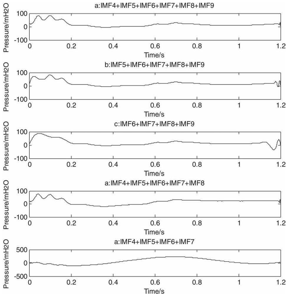
**Figure 8** | Reconstruction results of the IMF signals.
