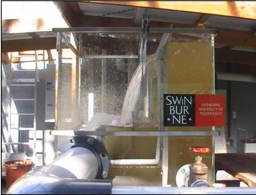
**Figure 2** | Set up of the Comb Separator.
