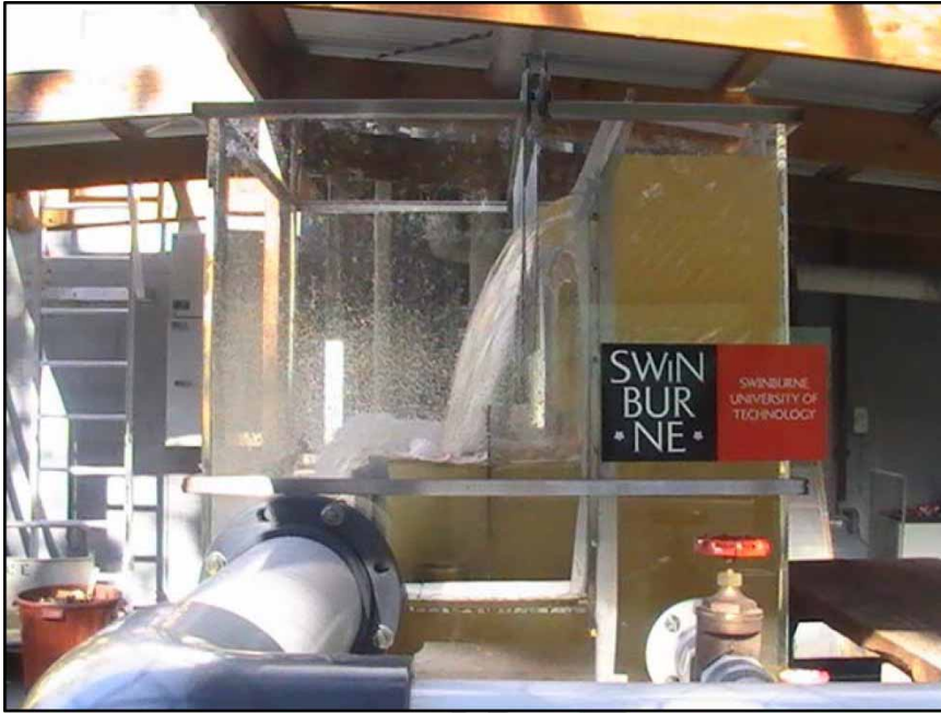
Figure 2 | Set up of the Comb Separator.
