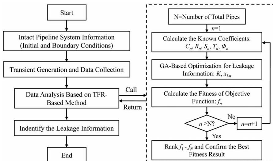
Figure 3 | Flowchart of TFR-based leak detection.
