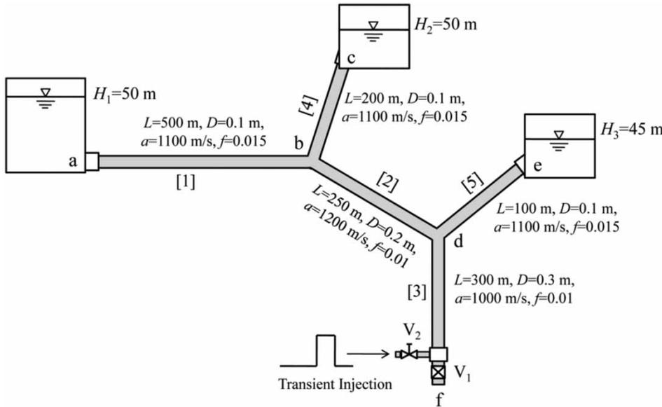
Figure 5 | Test pipeline system with two branched junctions.
