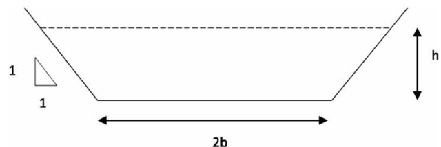
Figure 2 | Trapezoidal channel cross-section.
