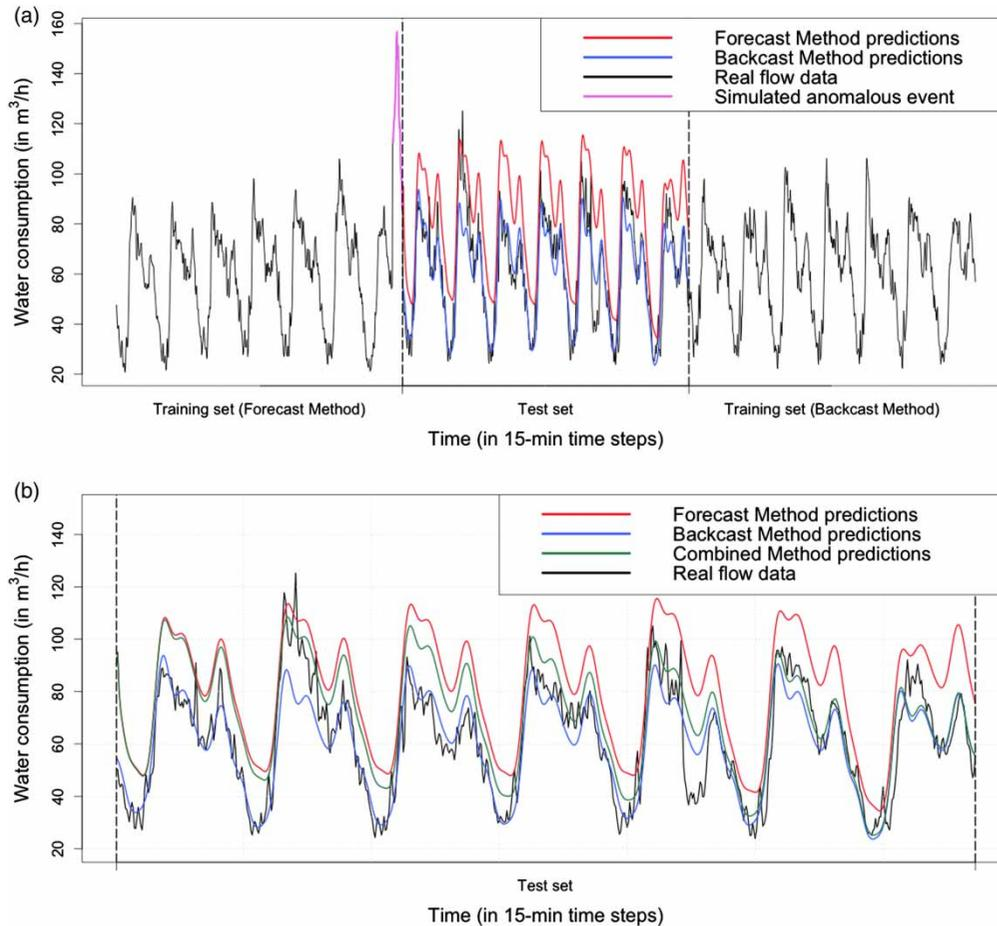
**Figure 8** | Forecast and Backcast Method predictions (a) and Combined Method predictions (b) with anomalous event.
