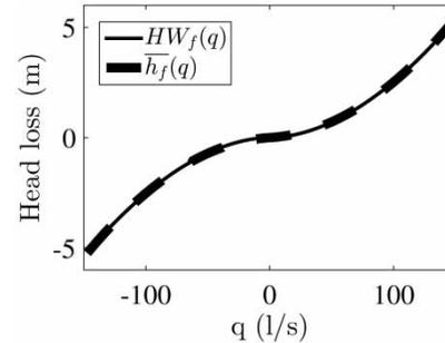
**Figure 1** | Graph of friction head loss computed using HW model and a quadratic approximation  $\bar{h}_f(q)$ . The considered pipe has  $L = 100$  m,  $D = 0.25$  m,  $C = 100$  and  $V^{\max} = 3$  m/s.
