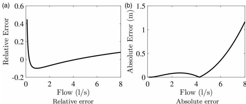
**Figure 3** | Graphs of relative and absolute error functions of the quadratic friction loss approximation for a typical pipe with L = 1,000 m, D = 0.1 m, C = 120. The value of Q<sub>2</sub> is set to 8 l/s while Q<sub>1</sub> is chosen so that the minimum of the relative error function ε<sub>rel</sub> sits at -0.1: (a) relative error, (b) absolute error.
