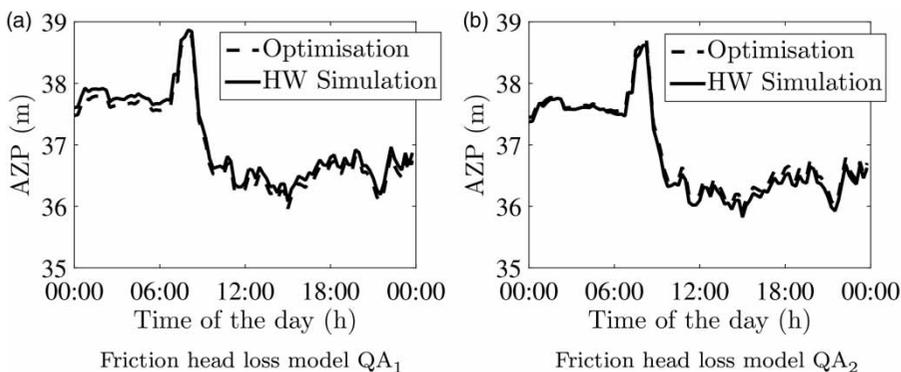
**Figure 13** | Comparisons of different AZP profiles obtained from optimisation and HW simulation: (a) friction head loss model QA<sub>1</sub>, (b) friction head loss model QA<sub>2</sub>.
