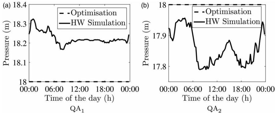
Figure 14 | Comparisons of pressure profile at the critical point for (a) QA<sub>1</sub> and (b) QA<sub>2</sub>.
