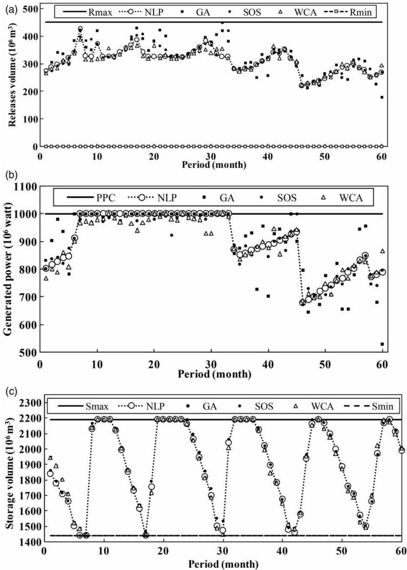
**Figure 8** | Comparison of the SOS algorithm, WCA, and the GA in their best performance for Karun4 reservoir problem in terms of (a) monthly release of the four-reservoir system and (b) power generated during the operational period, and (c) variations in storage volume.
