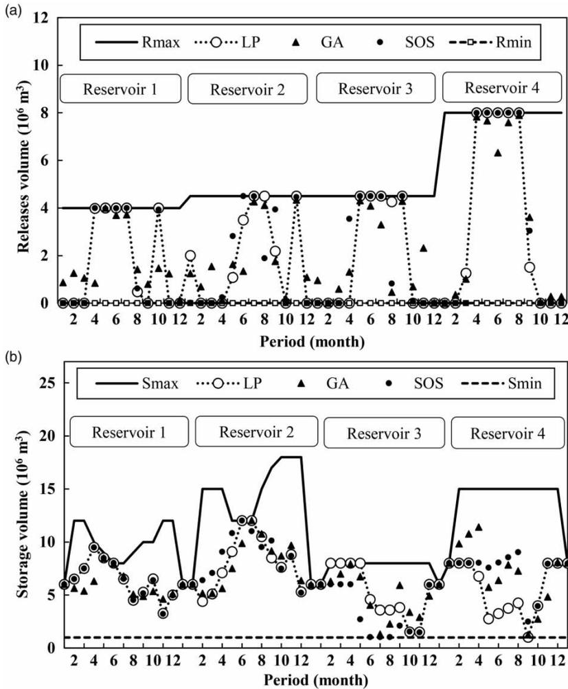
**Figure 6** | Comparison of the SOS algorithm, and the GA in their best performance for benchmark problem in terms of (a) monthly release of the four-reservoir system and (b) variations in storage volume.
