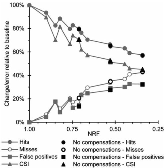
**Figure 9** | CSI of simplified models along with hits, misses and false positives. Hits and misses add up to 100% while false positives are excess pixels. Models without compensations are shown with black symbols for comparison.
