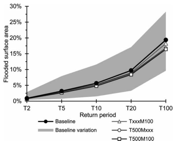
**Figure 7** | Flooded surface area as percentage of the total area of the mesh. The simplified models all underestimate the flooded area but do not exceed the reference variation computed via a 23% change in runoff from Hansen & Liu (2004).
