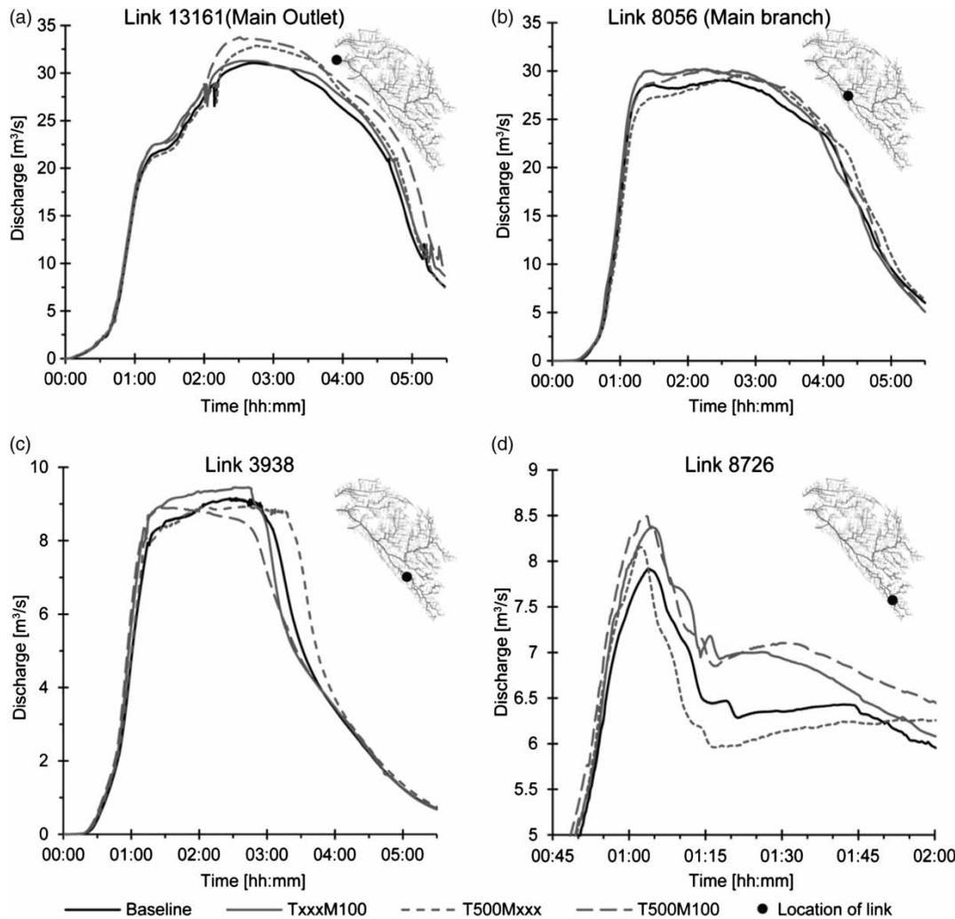
**Figure 5** | Hydrographs from the 1D hydraulic network model at a return period of 20 years for the baseline and most simplified models of the three approaches. The location of each link is indicated by a black dot on the small map in the top right of each sub-figure.
