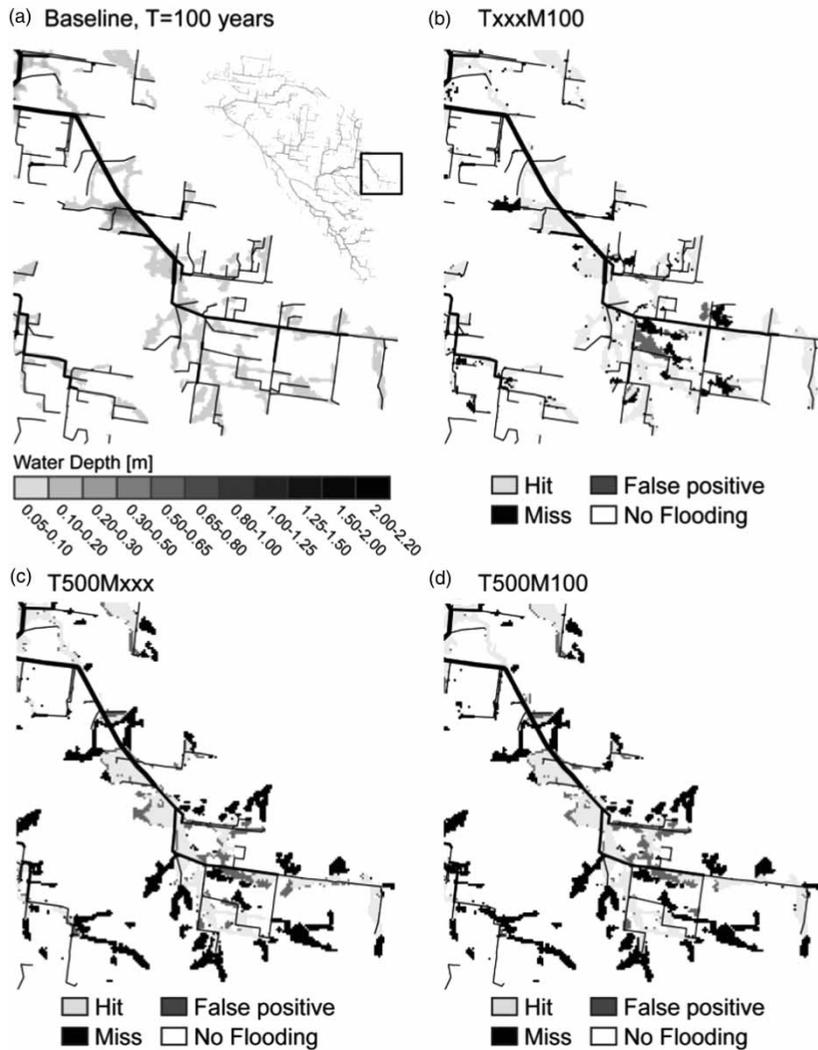
**Figure 8** | (a) An overview with the maximum water depth for the baseline during a 100-year event. (b)–(d) The differences from the baseline in spatial flood results for the TxxxM100, T500Mxxx and T500M100 models, respectively.
