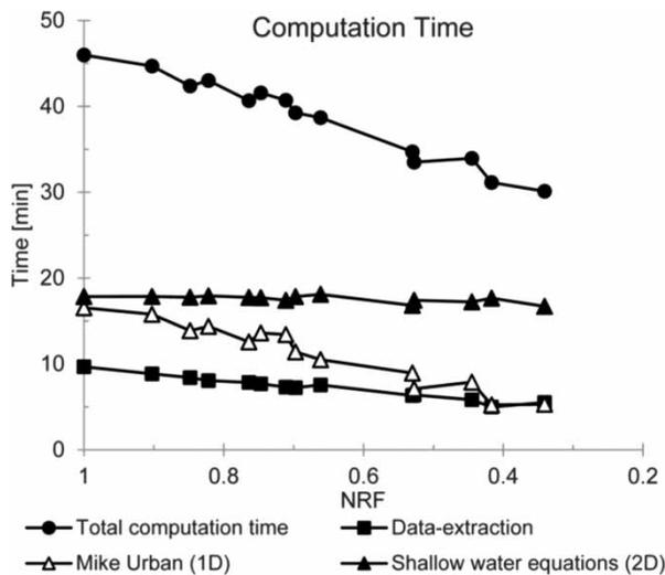
**Figure 4** | Computation time of the baseline and simplified models. The computation time depends on the number of model elements, hence the network reduction factor (NRF) is used for the horizontal axis. The computation time decreases with the number of elements in the 1D hydraulic network model due to both faster 1D calculations and fewer data to load and save during simulations. The 2D computation time is constant for all models.
