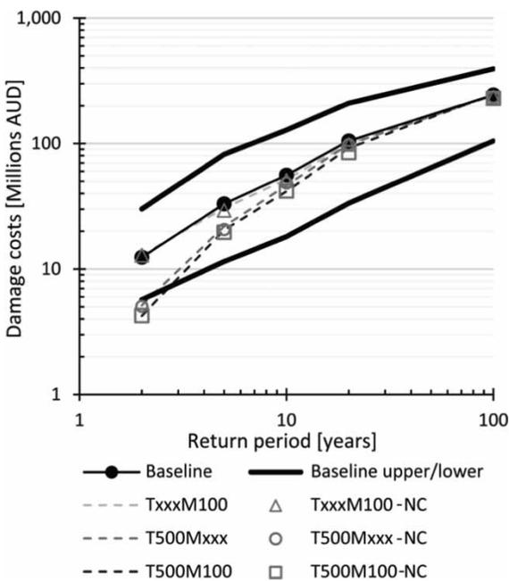
**Figure 10** | Total damage costs of flooding for selected models. The baseline variation indicates the variation of the costs by changing the runoff only, i.e., the uncertainty of the valuation of the damages is not included.
