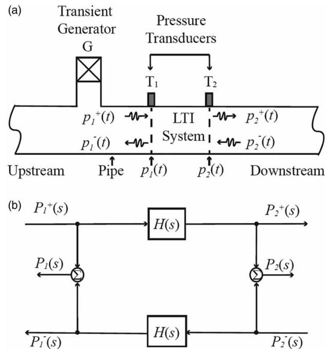
**Figure 1** | (a) Proposed configuration for the pressure transient test with a dual-sensor in a pipeline; and (b) corresponding block diagram in the frequency domain illustrating the wave propagation (LTI System = Linear Time Invariant System).
