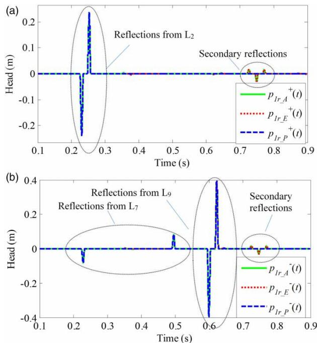
**Figure 4** | (a) Directional reflected pressure waves travelling from upstream to downstream; and (b) directional reflected pressure waves travelling from downstream to upstream.
