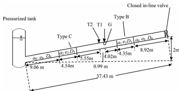
Figure 5 | System layout of the experimental pipeline system.
