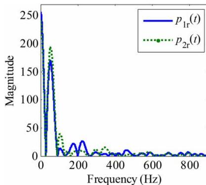
Figure 7 | Amplitude spectrum of the reflected waves.
