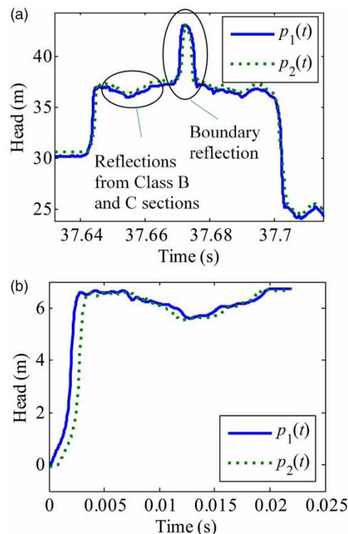
Figure 6 | (a) Original pressure traces measured in the laboratory experiments; and (b) pressure oscillations before the first boundary reflection.
