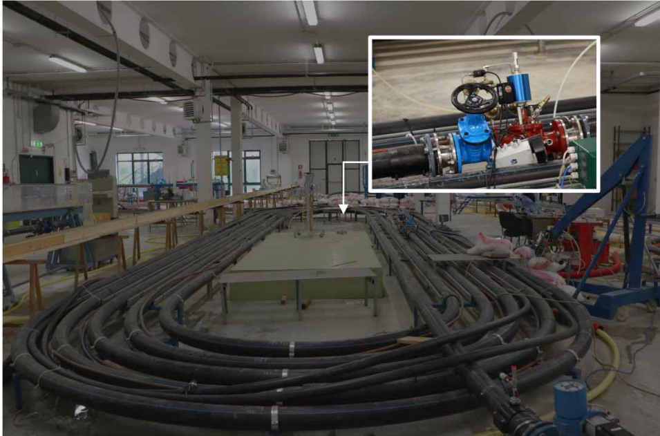
Figure 2 | The experimental pipe and the PRV (in the insert) at the Water Engineering Laboratory (WEL) of the University of Perugia, Italy.
