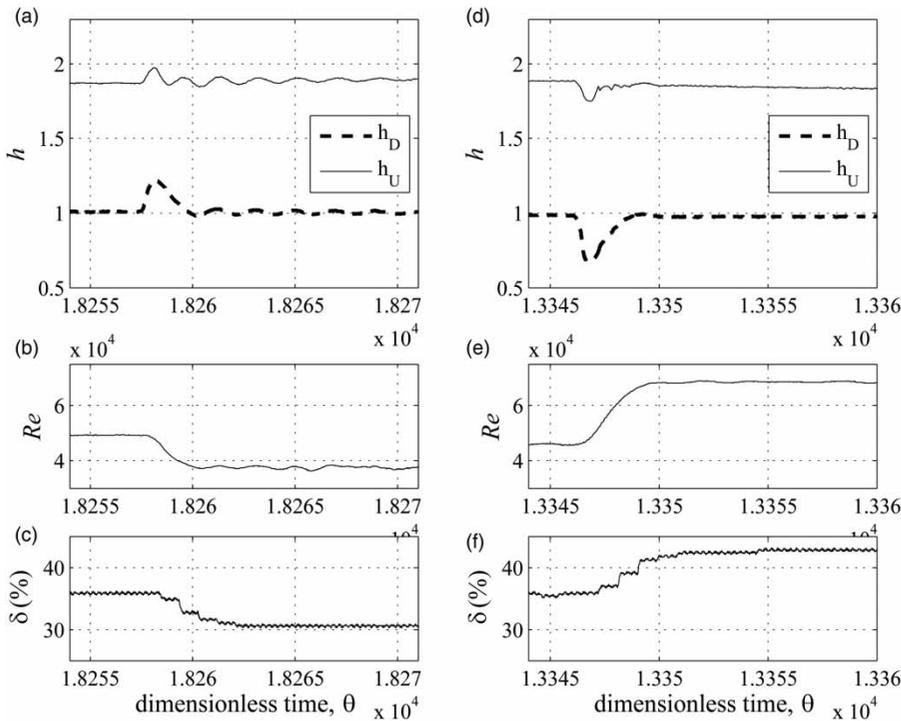
Figure 12 | Long duration transient (test no. 13): magnified vision of Figure 11 in the time interval when the largest demand decrease (a)–(c) and increase (d)–(f) take place, respectively.
