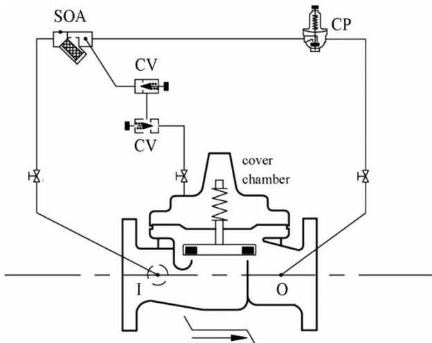
**Figure 3** | Schematic of the PRV (modified from <http://www.cla-val.com/waterworks-pressure-reducing-valves>): I = inlet section, O = outlet section, CV = check valve, SOA = strainer-orifice assembly, CP = control pilot.
