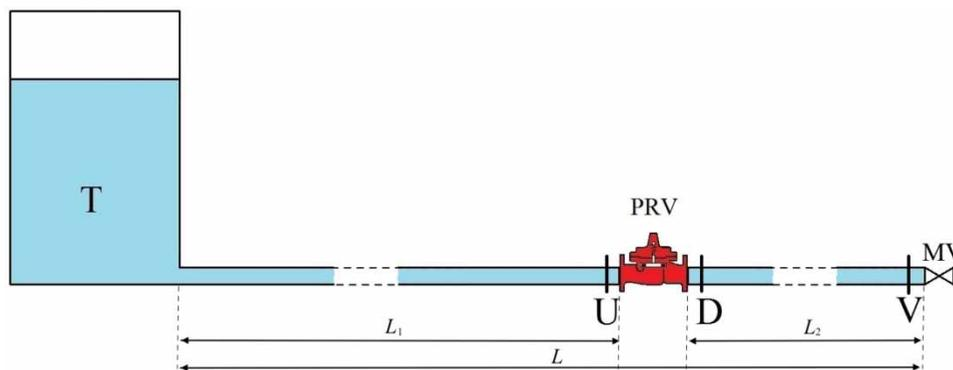
**Figure 1** | Sketch of the experimental setup (T = supply tank; PRV = pressure reducing valve; MV = manoeuvre valve; pressure measurement sections: U = upstream of the PRV; D = downstream of the PRV; V upstream of the MV).
