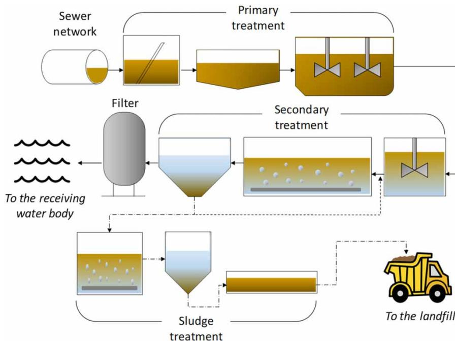
Figure 2 | The analysed integrated urban wastewater system outline.
