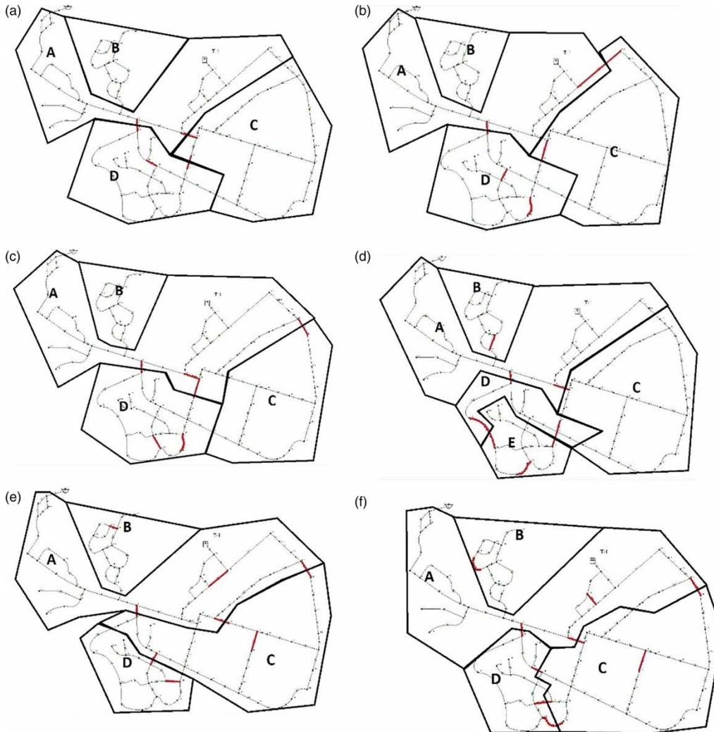
**Figure 5** | DMAs' formations for the scenarios tested: (a) 4 pipes closed scenario; (b) 5 pipes closed scenario; (c) 6 pipes closed scenario; (d) 7 pipes closed scenario; (e) 8 pipes closed scenario; and (f) 9 pipes closed scenario.
