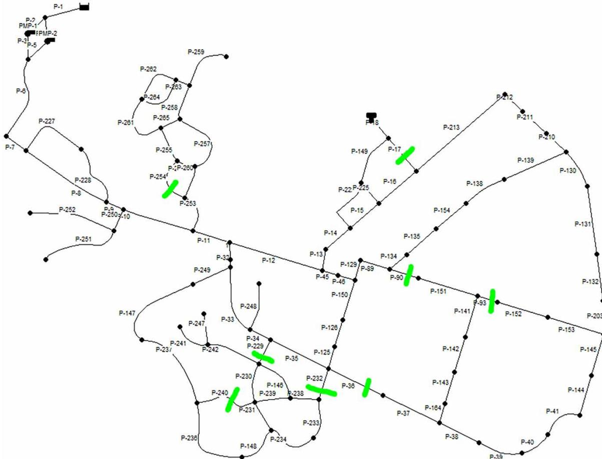
**Figure 2** | Closed pipes highlighted with a strikethrough grey line.
