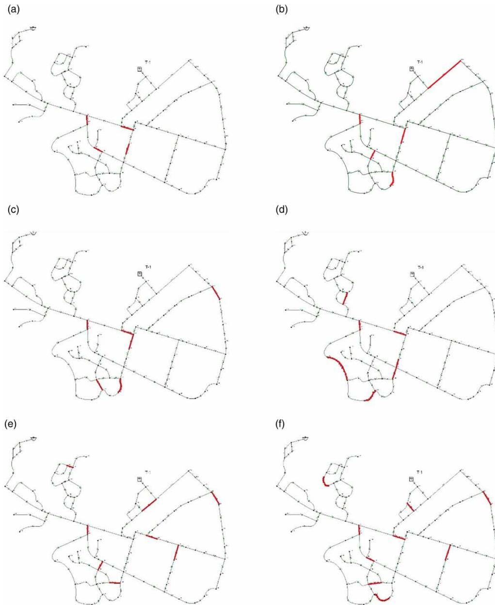
**Figure 4** | Optimal closed pipes configurations for each scenario (closed pipes in bold lines): (a) 4 closed pipes scenario; (b) 5 closed pipes scenario; (c) 6 closed pipes scenario; (d) 7 closed pipes scenario; (e) 8 closed pipes scenario; and (f) 9 closed pipes scenario.
