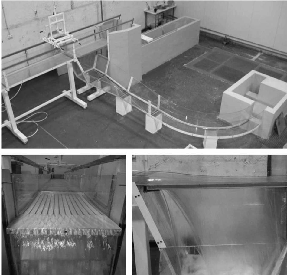
**Figure 4** | Intake system physical device.
