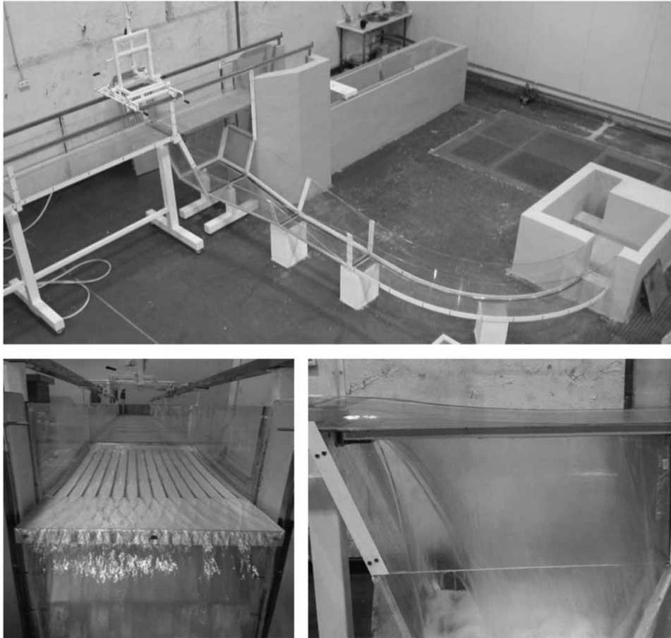
Figure 4 | Intake system physical device.
