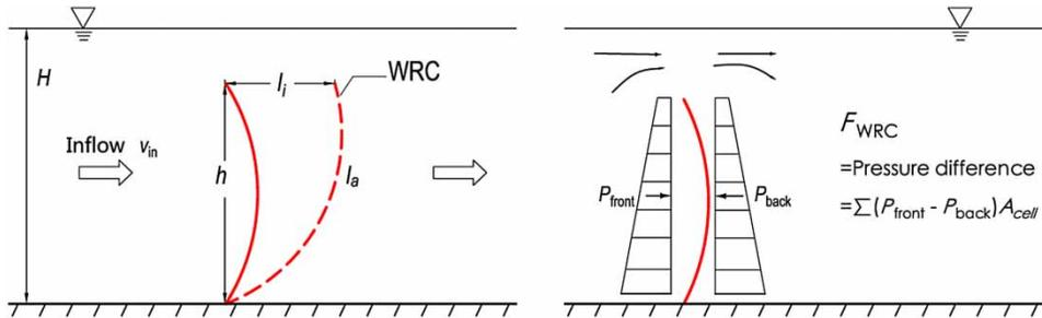
**Figure 1** | Sketch of the thrust and arrangement form of a WRC, where  $v_{in}$  is inflow velocity,  $H$  is water depth,  $h$  is water-retaining height,  $l_a$  is arc length,  $l_i$  is inclination length,  $F$  is the force of WRC,  $P$  is pressure, and  $A_{cell}$  is area of the curtain cells.
