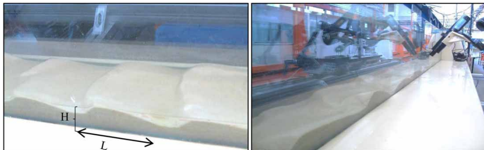
Figure 3 | Dune bedform geometry (Roushangar 2010).
