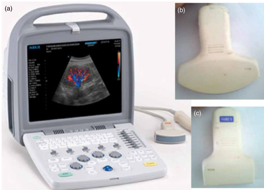
Figure 1 | B-mode ultrasound device: (a) the mainframe, (b) the convex probe, and (c) the linear probe.
