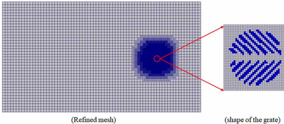
Figure 4 | Mesh characterisation example for grate type A.
