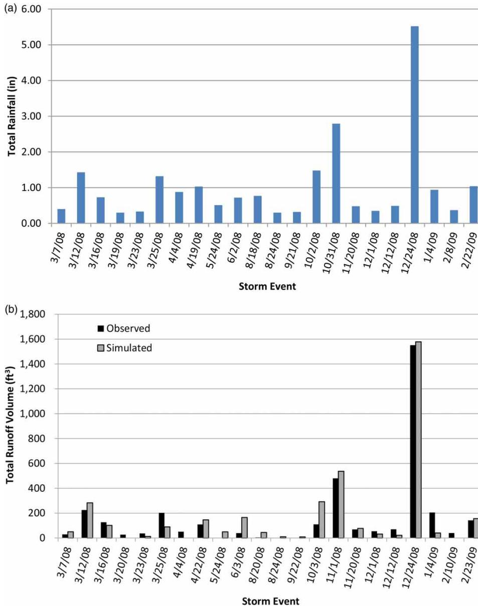
**Figure 4** | (a) Total rainfall variation for 22 events used for validation procedure. (b) Comparison of observed and simulated total runoff volume in the validation procedure considering evapotranspiration.
