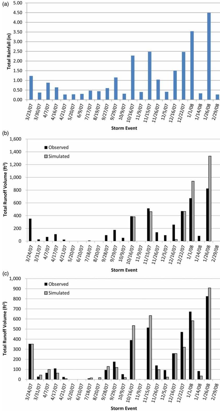
**Figure 3** | (a) Total rainfall variation for 23 events used for calibration procedure. (b) Comparison of observed and optimal simulated total runoff volume in the calibration procedure without consideration of evapotranspiration. (c) Comparison of observed and optimal simulated total runoff volume in the calibration procedure considering evapotranspiration.
