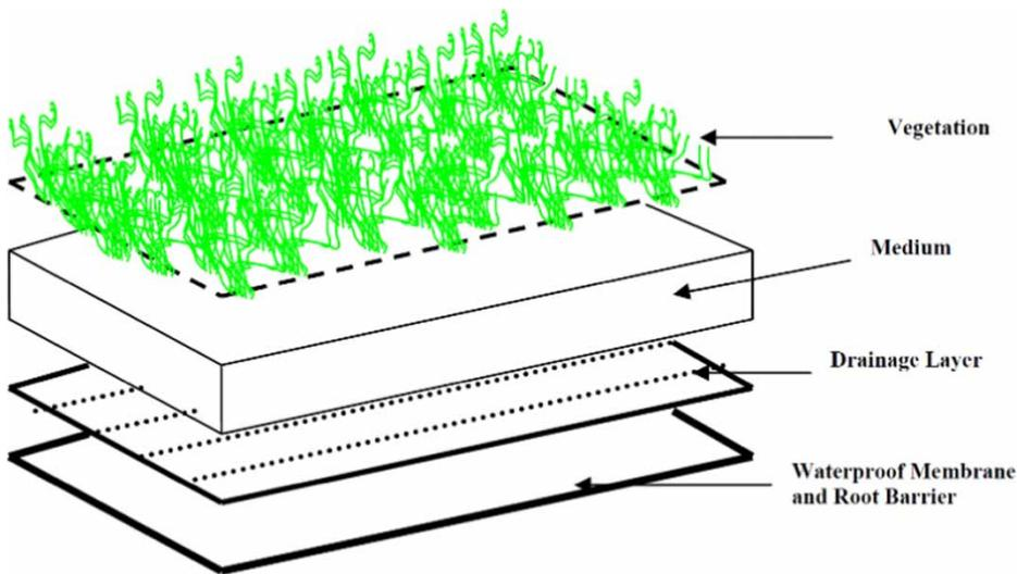
**Figure 1** | Typical cross-section of a green roof system (Berghage *et al.* 2009).
