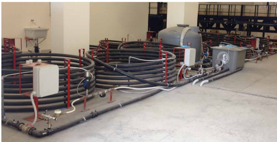
Figure 1 | Top: Layout of the experimental WDN. Bottom: Overview of the WDN.
