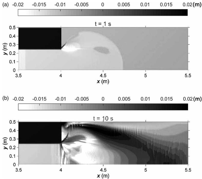
**Figure 3** | Computed bed change compared to the original bed at (a)  $t = 1$  s; (b)  $t = 10$  s.
