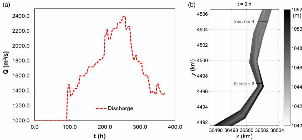
**Figure 10** | Inflow hydrograph (a) and the initial bed elevation (b) at the Bayangaole Reach of Yellow River.
