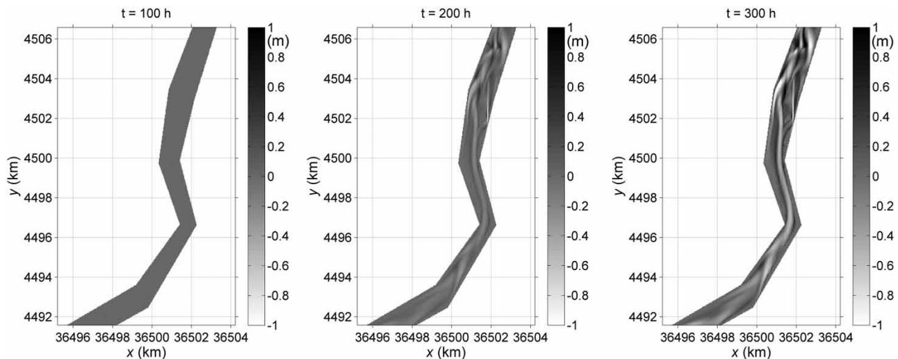
Figure 15 | Computed bed change compared with the original at the Bayangaole Reach of Yellow River for a following flood event.
